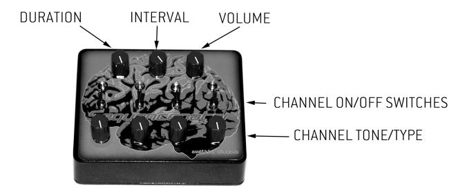
EACH OF THE FOUR STEPS PRODUCES A NOTE IN TURN. YOU CAN ADJUST THE TIMBRE AND TYPE OF NOTE WITH EACH OF THE CHANNEL'S TONE KNOB. WHEN THE KNOB IS TURNED TO THE LEFT OF CENTER, THAT CHANNEL WILL PRODUCE TWEAKABLE WHITE NOISE — AND TUNABLE BLEEP TONES TO THE RIGHT OF CENTER.
