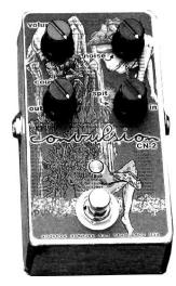
NOISE knob — mixes white noise with the input signal COUGH knob — adjusts the amount of oscillation SPIT knob — adjusts sound decimating VOLUME knob — adjusts the audio level of the final output
